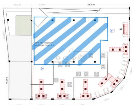
Fig. 11. Marked area (blue) without AC unit.
