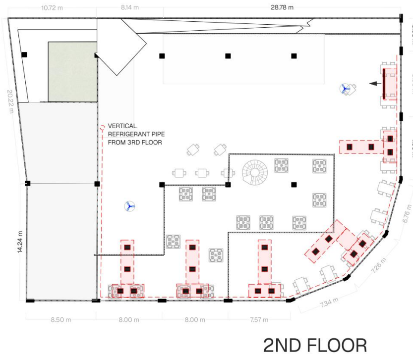
Fig. 5. VRV units and ceiling fans mapping.
